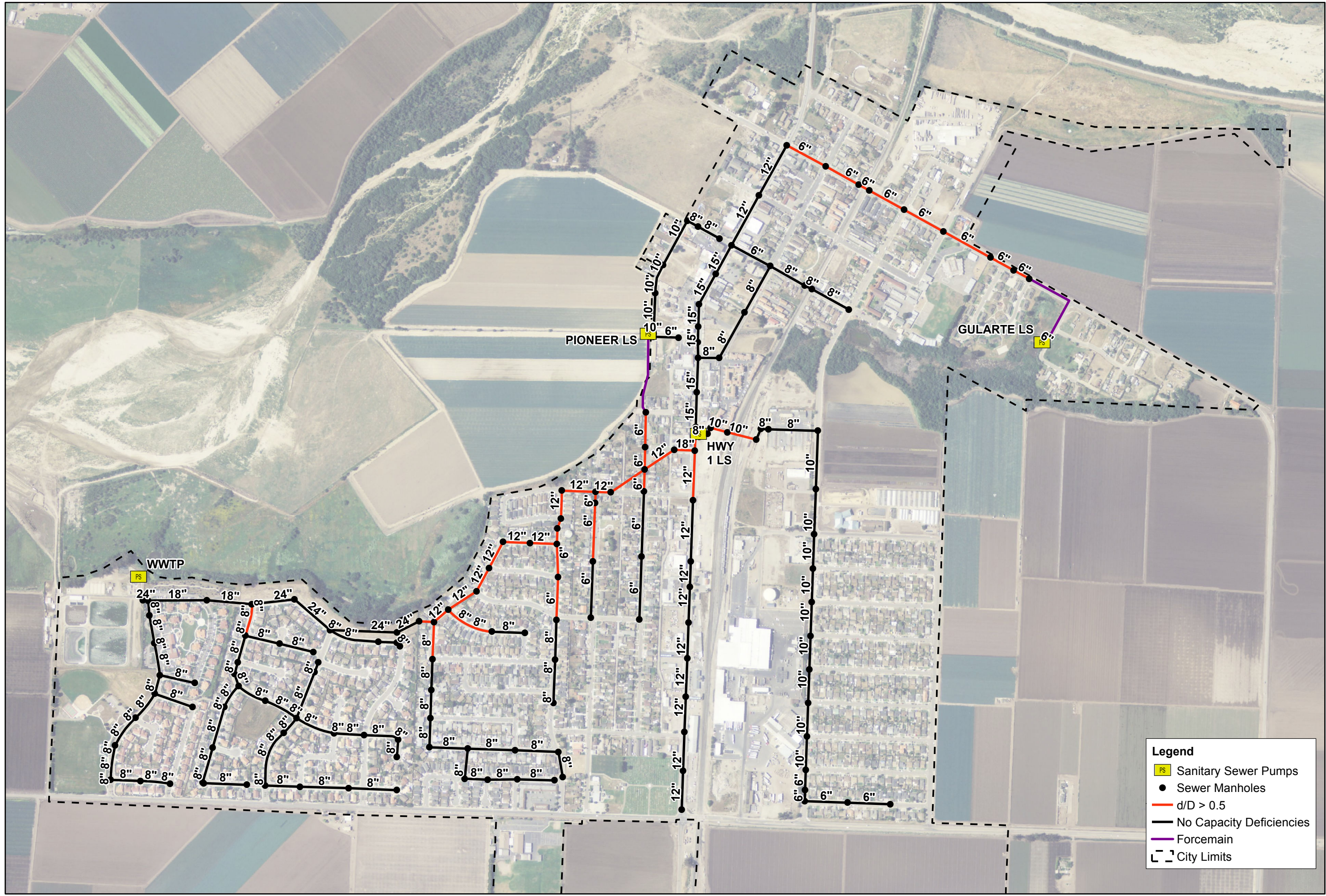
Figure 6-3: Existing ADF Collection System Deficiencies
