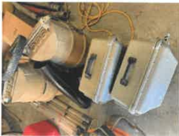
Composite Samplers: do not operate, cannot get parts for two of them and the other two not needed even for spare parts, a fifth sampler, black, not pictured, is also obsolete. City has a new composite sampler. Sludge judges are also in the picture: not needed, Not the right size, have newer replacements.
