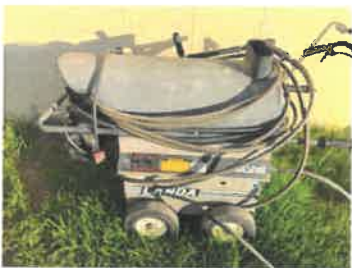
Heated Pressure washer: still operates but needs repair, rusty, City has a smaller more useful pressure washer.
