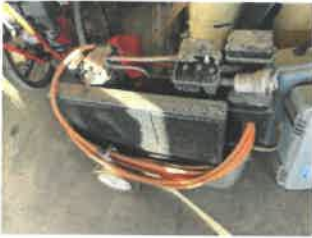
Air compressor: would not turn on at all, really old, City has a newer electric compressor.
