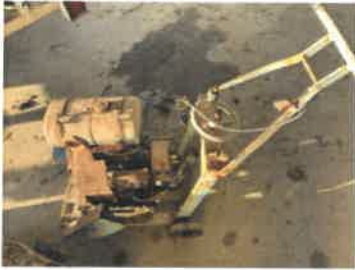
Concrete cutter: too old to operate safely.
