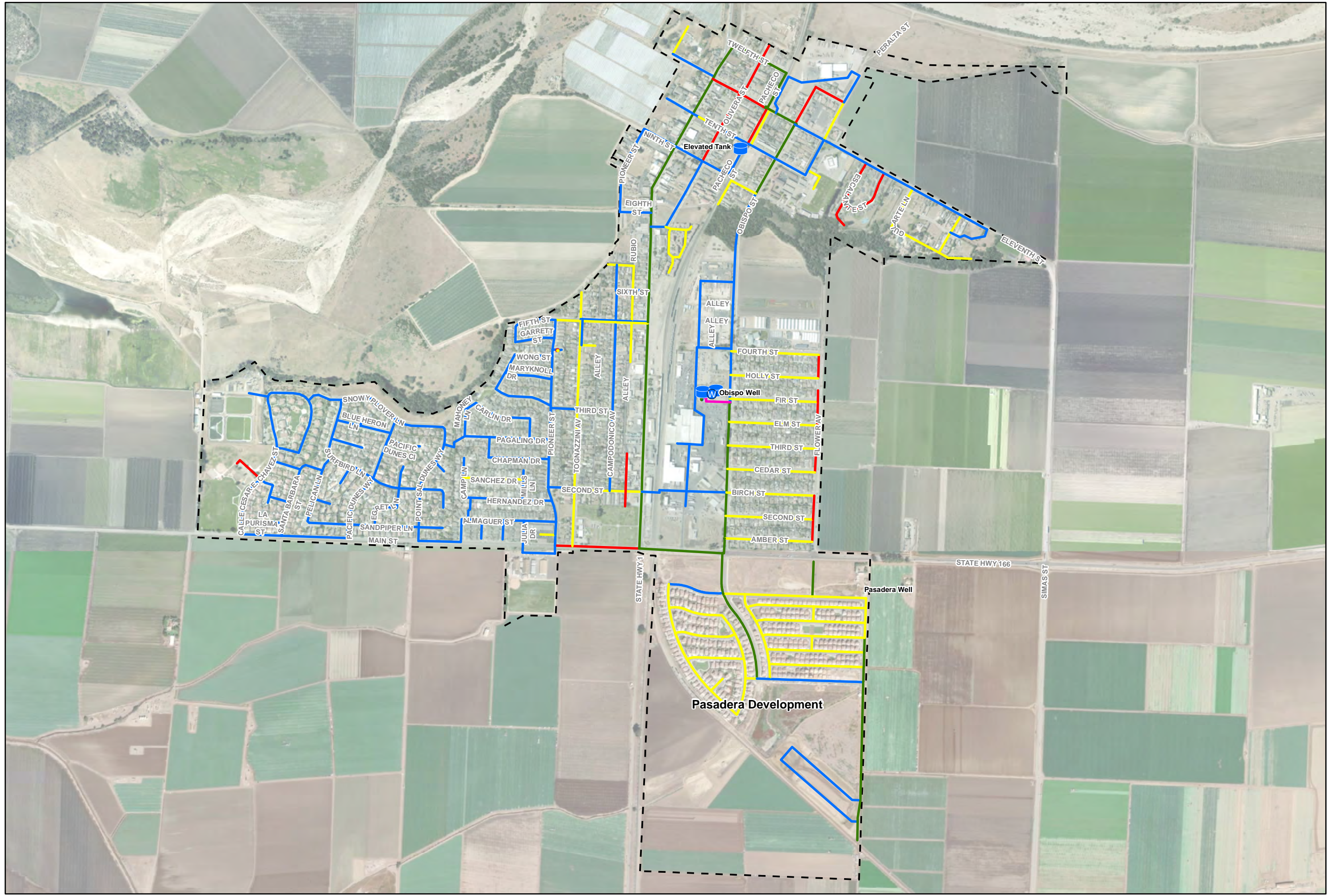
Figure 4-1: Existing Water Distribution System
